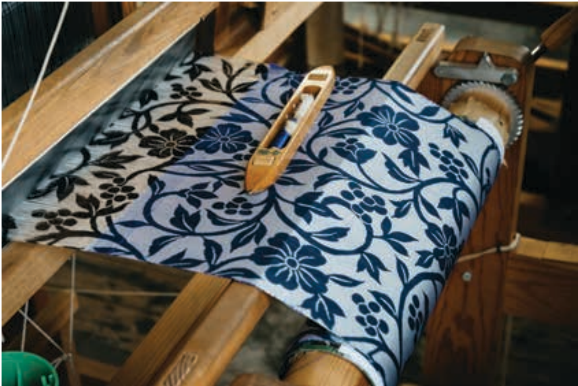
Figure 3.10 Meisen on loom: showing stencil-dyed warp threads.
